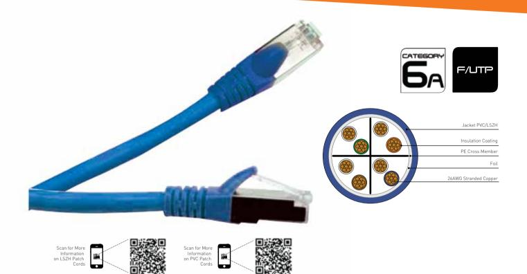
Category  $6_A$  Foiled Twisted Pair (F/UTP) patch cords conform to class EA standards. Our patch cords are made to the highest standards, using only quality stranded cable, giving you the best in flexibility, plus top grade 50µ gold plated RJ45 connector plugs for high quality connections. This combination makes for outstanding performance and reduced degradation. Aluminium tape is used to shield all 4 pairs; this gives a screened protection against external interference such as EMI.
